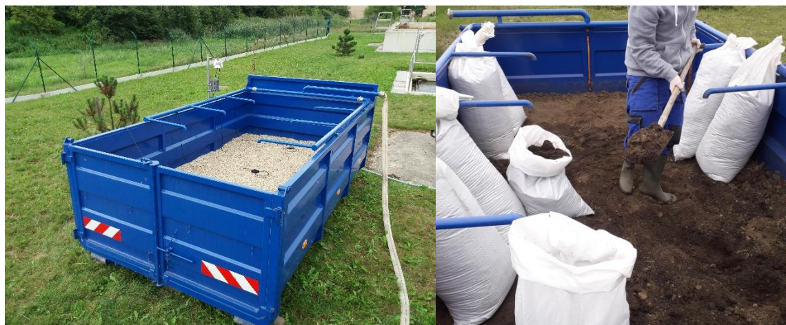
Figure 4: Mobile RB unit at the beginning of the operation on the left and during the excavation of dewatered and stabilized sludge on the right
