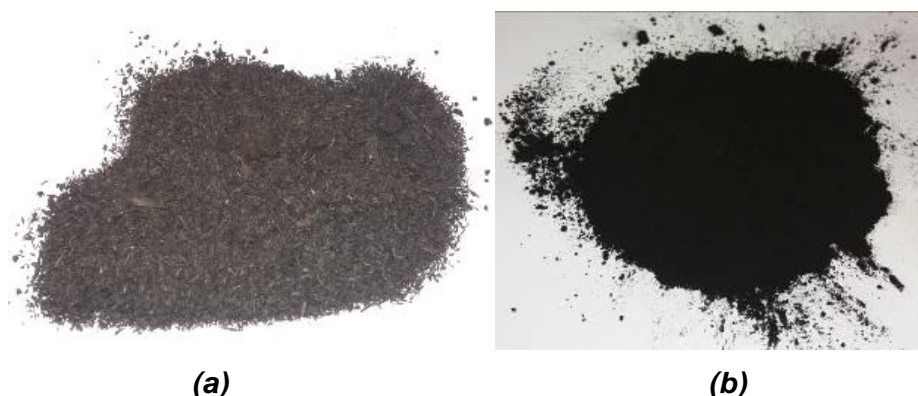
Figure 2: Digestate (a) after drying and milling, and (b) after pyrolysis at 300 °C (biochar)
