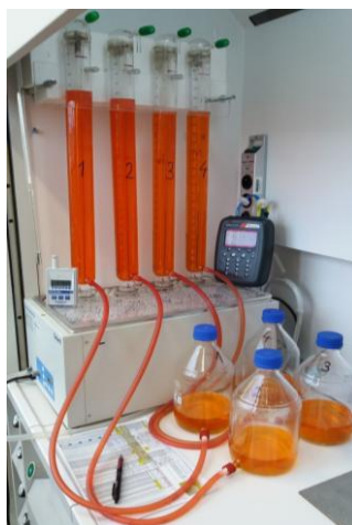
Figure 3: Experimental unit for BMP tests
